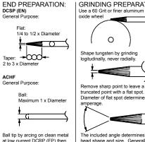
Shape tungsten by grinding Remove sharp point to leave a truncated point with a flat spot. Diameter of flat spot determines The included angle determines weld bead shape and size. Generally, slowly increase current to form as the included angle increases. the desired ball diameter. penetration increases and bead
